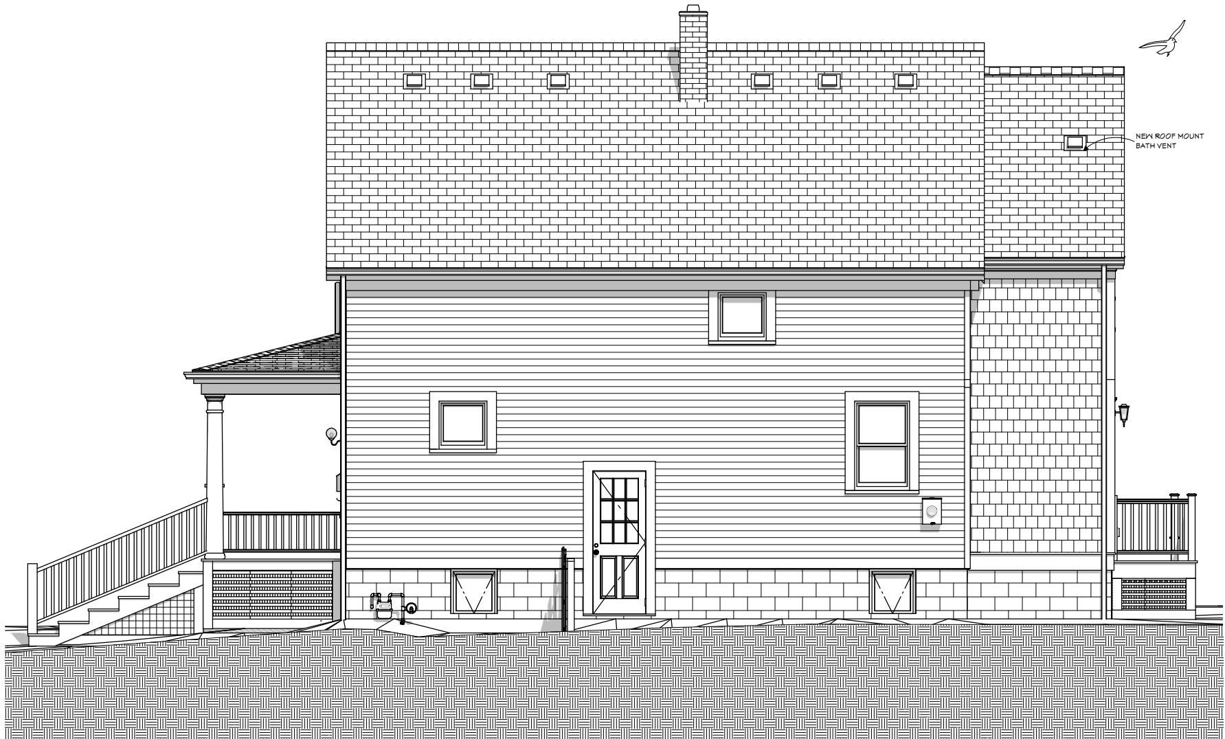
SIDE ELEVATION (EAST) - PROPOSED SCALE: 5/32" = 1'-0"
