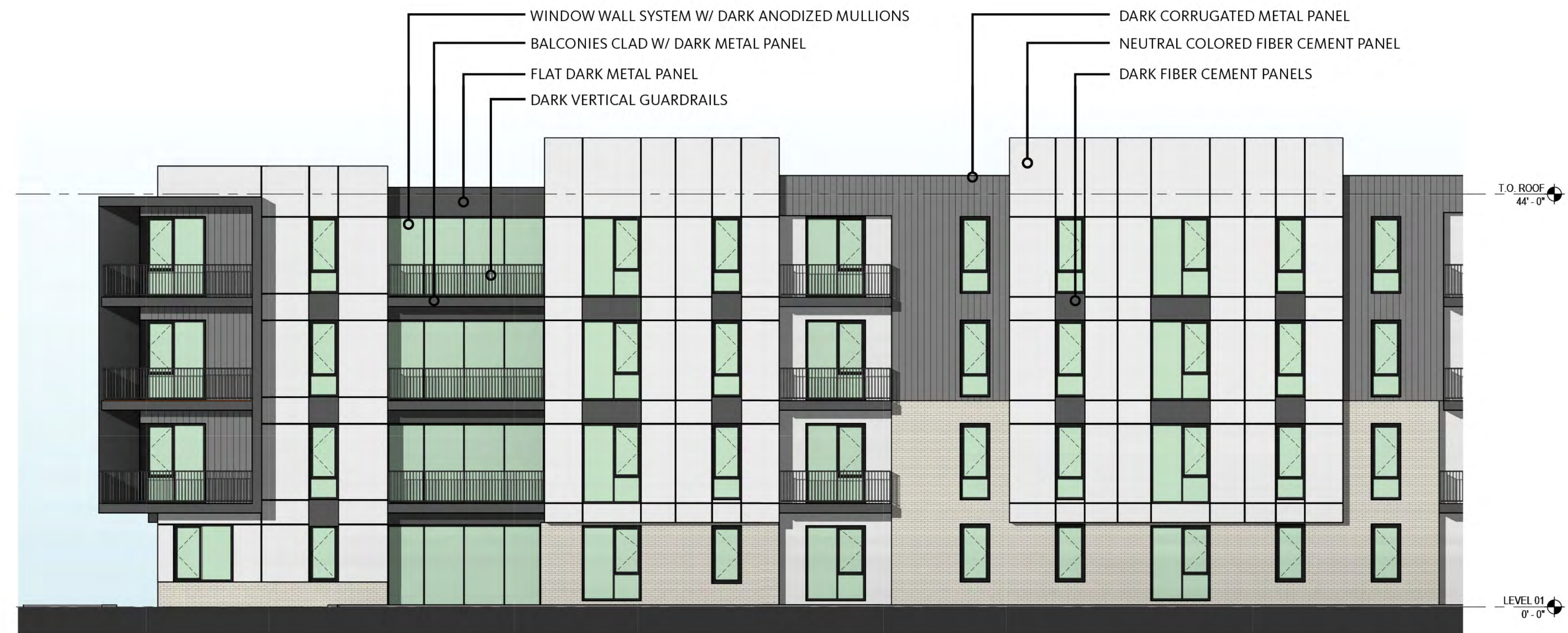
ENLARGED EXTERIOR EAST ELEVATION
