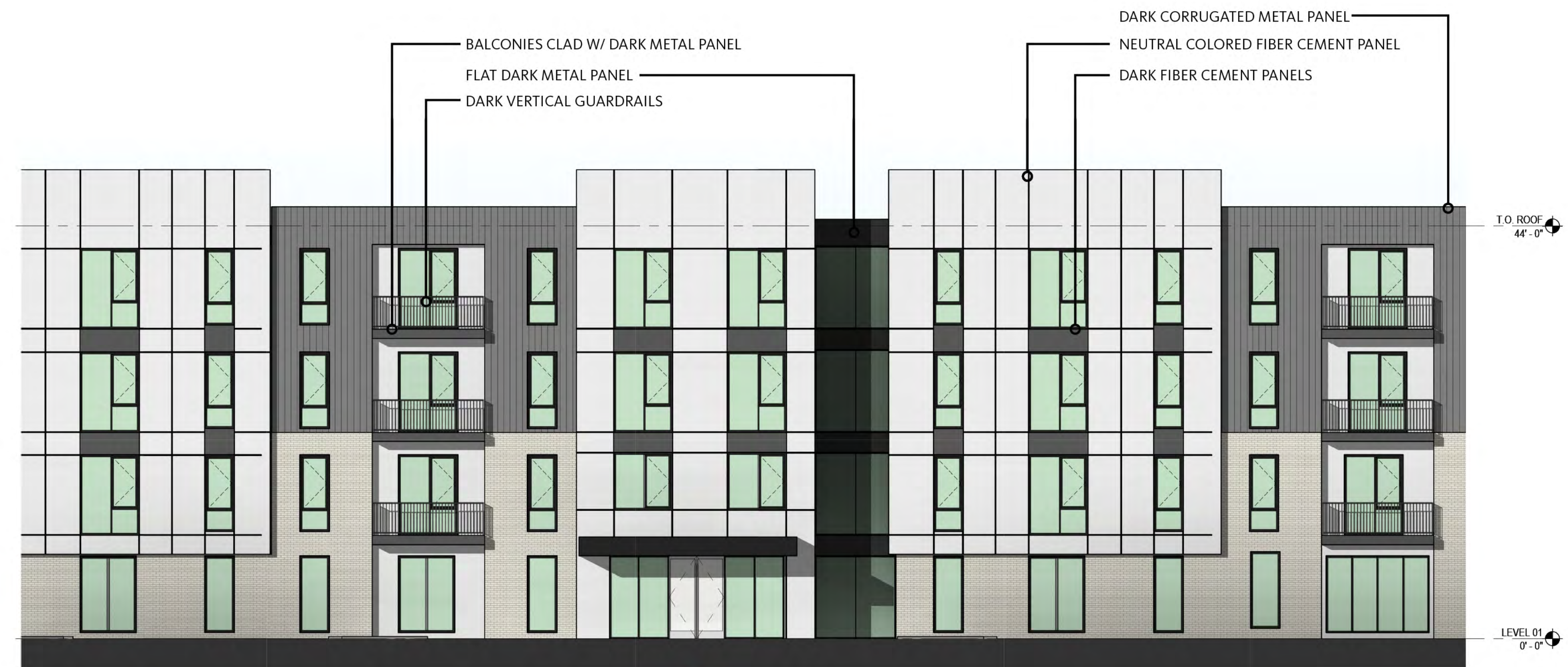
ENLARGED EXTERIOR EAST ELEVATION
