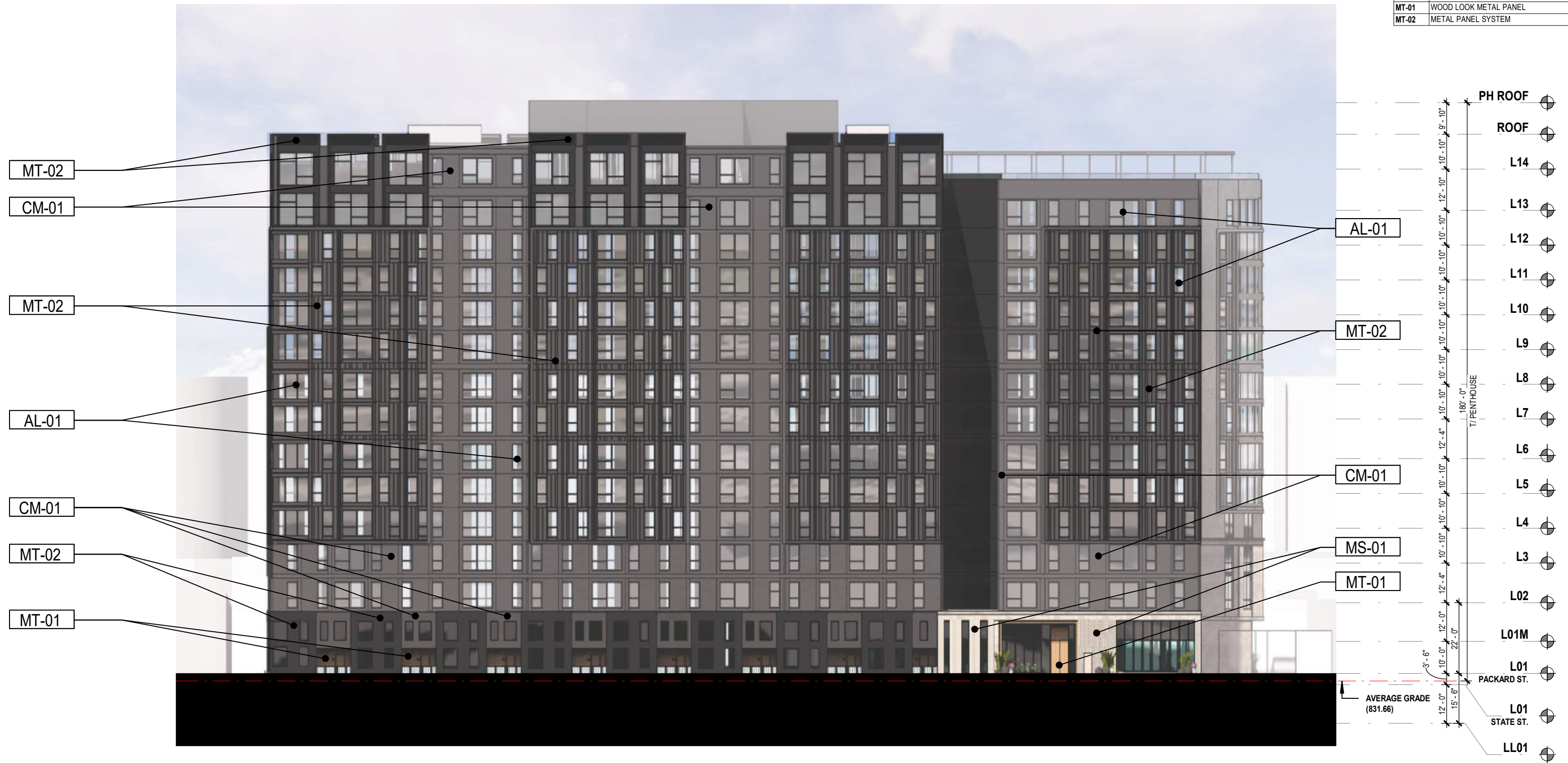
1 EXTERIOR BUILDING ELEVATION - EAST P3.1 SCALE: 1" = 30'-0"
