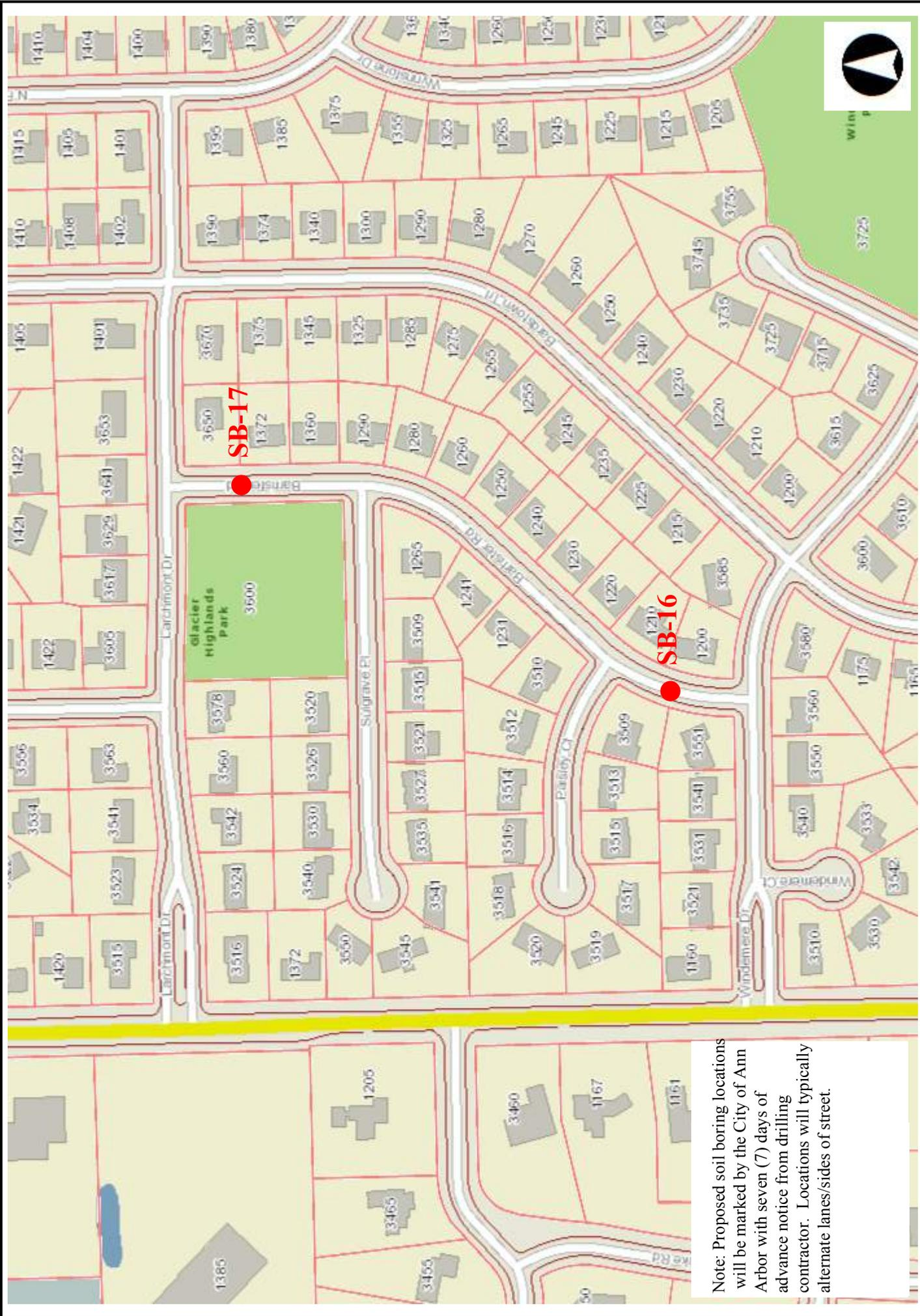
Note: Proposed soil boring locations will be marked by the City of Ann Arbor with seven (7) days of advance notice from drilling contractor. Locations will typically alternate lanes/sides of street.
