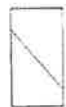
Type 4 Diagonal fracture with no crack going through base (add a 2nd arrow to distinguish from Type 1)
