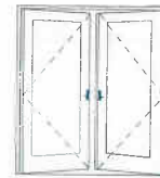
FWH 6058 A P L R Frenchwood™ Hinged Inswing Patio Door Active Panel Left Hinged Door Rough Opening Passive Panel Right Hinged
