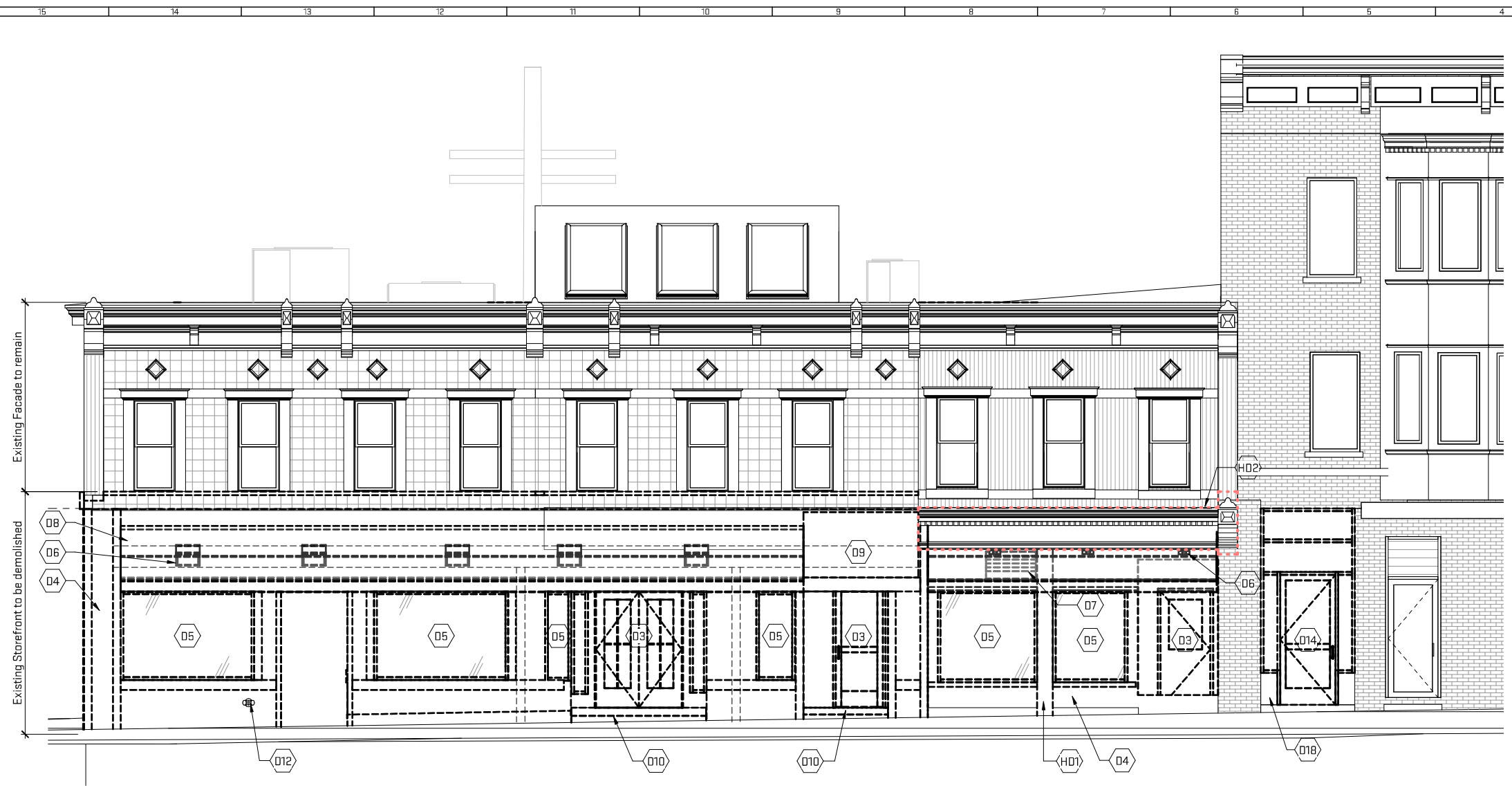
1 South Elevation - Proposed Storefront Demolition AD-101 1/4" = 1'-0"
