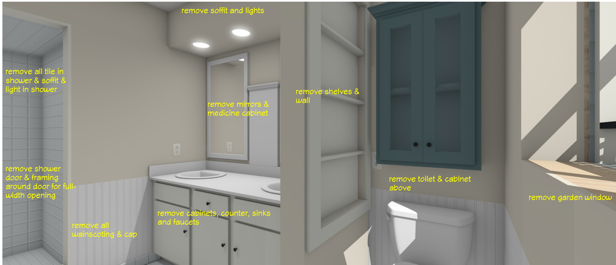
MASTER BATH TEAROUT PLAN SCALE 1/2"=1'0" 8'-10" X 6'-3"
