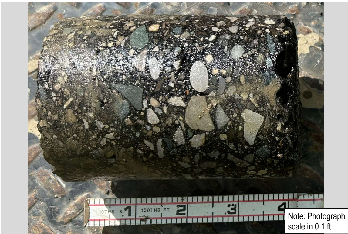
Photo 13: SB-2026-120 (Packard St.): 5-inch Asphalt
