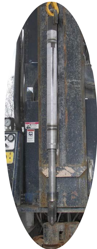
Push Ahead Vertical Aquifer Sampler
