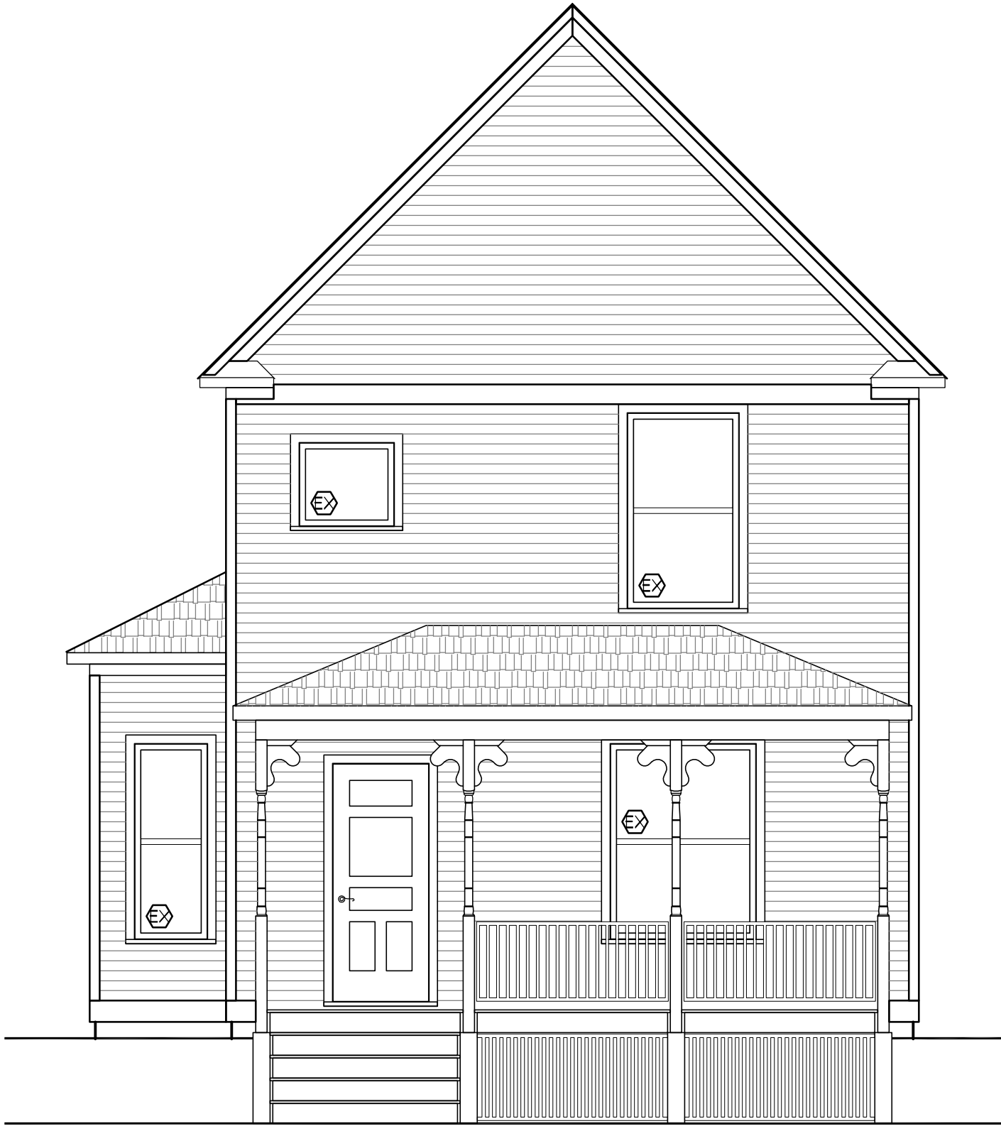
1 FRONT (SOUTH) ELEVATION – EXISTING A-9 SCALE: 1/4" = 1'-0"
