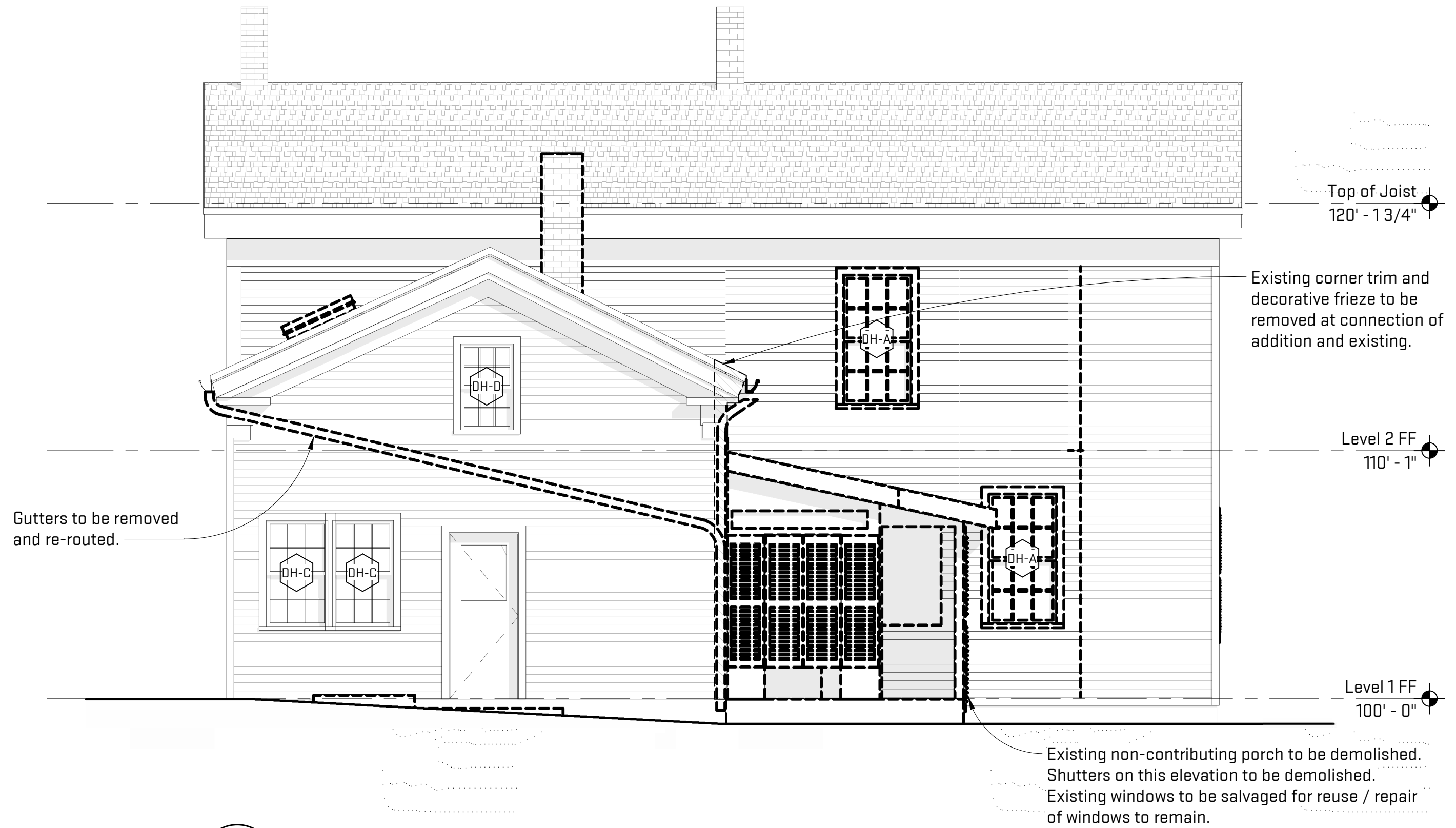
2 North Elevation - Existing A-302 1/4" = 1'-0"
