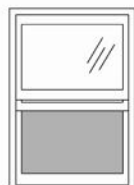
Shaded portion shows vent area.
