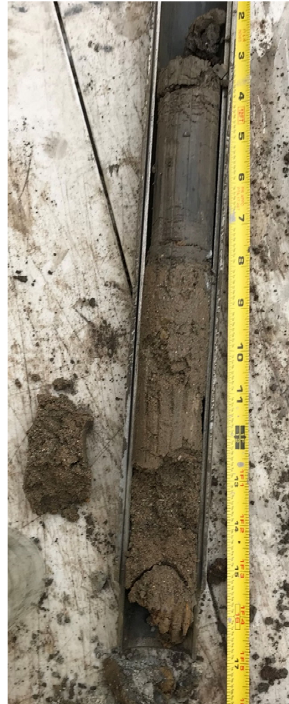
Figure 2: TB-2 S-5, granular soil present at about 14 feet deep
