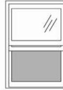
Shaded portion shows vent area.
