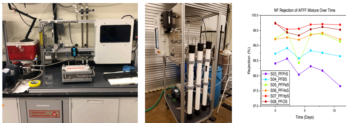
Figure 4. (Left) bench-scale membrane system at CSM, (middle) pilot-scale membrane system at CSM, (right) rejection of PFAS as a function of time by NF270.
