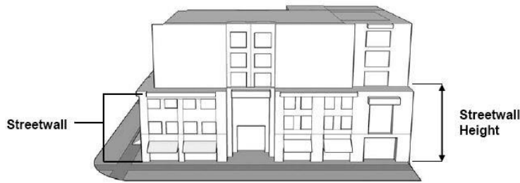
Figure 5 - Streetwall and Streetwall Height
