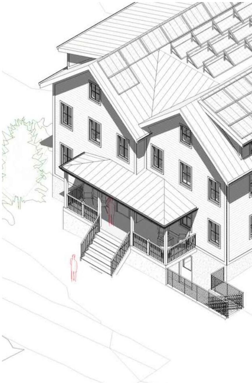
ORIGINAL DESIGN – STAIRS REQUESTED TO MOVE TOWARD HOUSE AND REMOVE HANDRAIL
