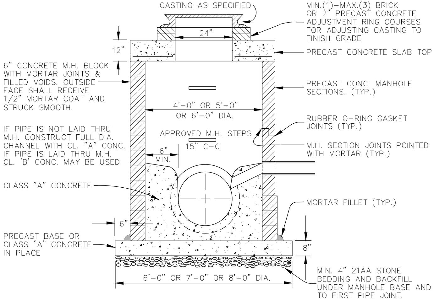
6" CONCRETE M.H. BLOCK WITH MORTAR JOINTS & FILLED VOIDS. OUTSIDE FACE SHALL RECEIVE 1/2" MORTAR COAT AND STRUCK SMOOTH.
