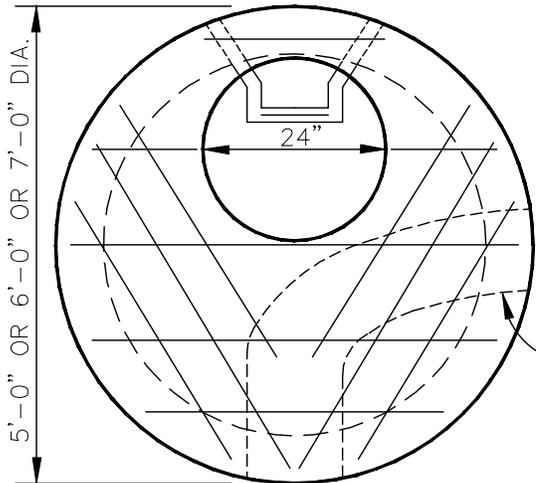
TO BE CONSTRUCTED FOR STORM OR SANITARY SEWERS IF STANDARD M.H. CAN NOT BE BUILT DUE TO LACK OF COVER.
