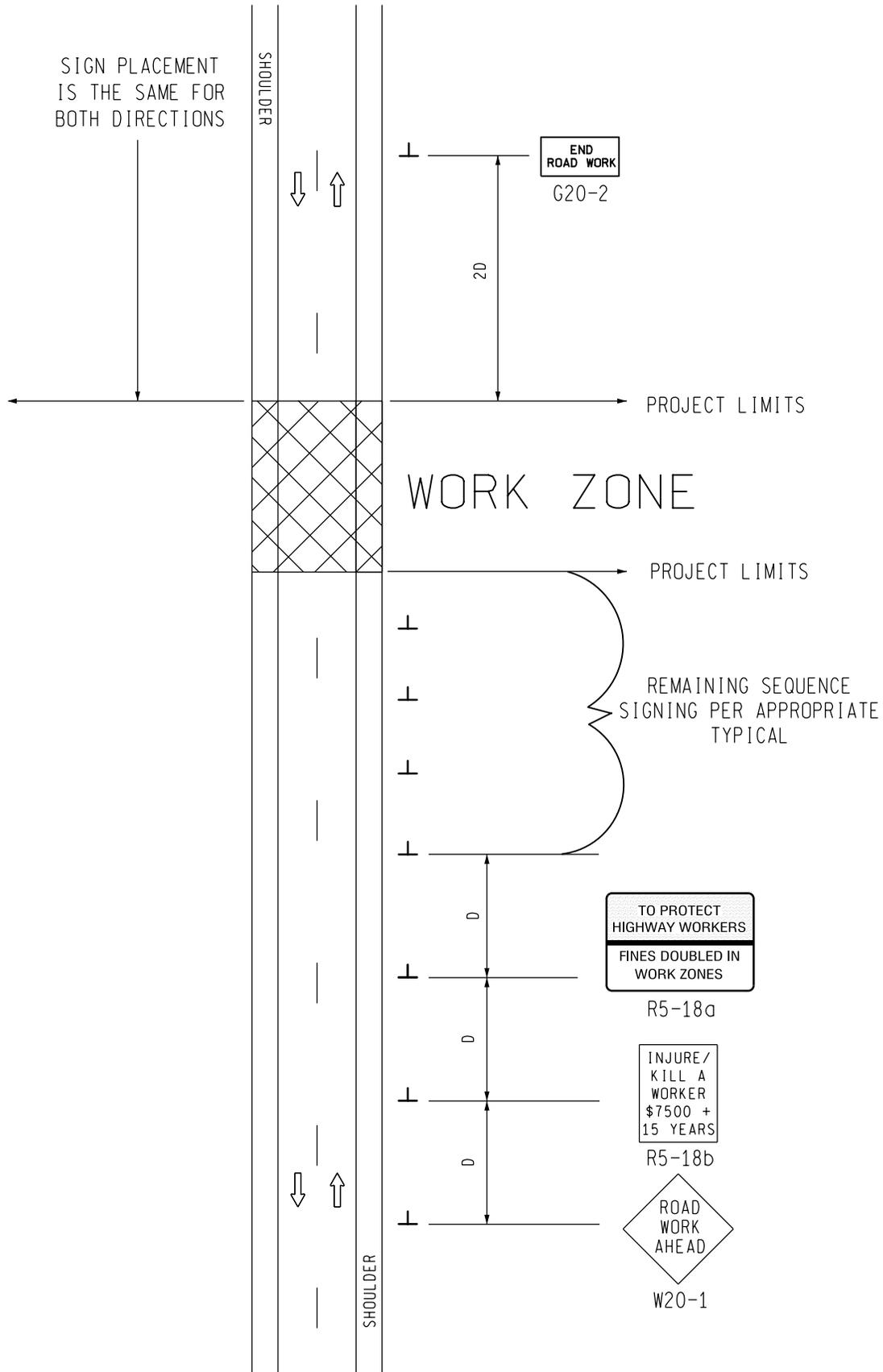
SIGN = 68 f+2 - TYPE B FOR ONE DIRECTION OF TRAFFIC W20-1 QUANTITY INCLUDED WITH APPROPRIATE TYPICAL FOR SEQUENCE SIGNING
