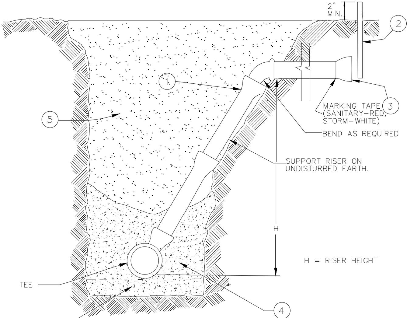
NOTE: A TEE SHALL BE USED AT THE SEWER MAIN IF A RISER IS USED. WYES ARE NOT TO BE USED.
