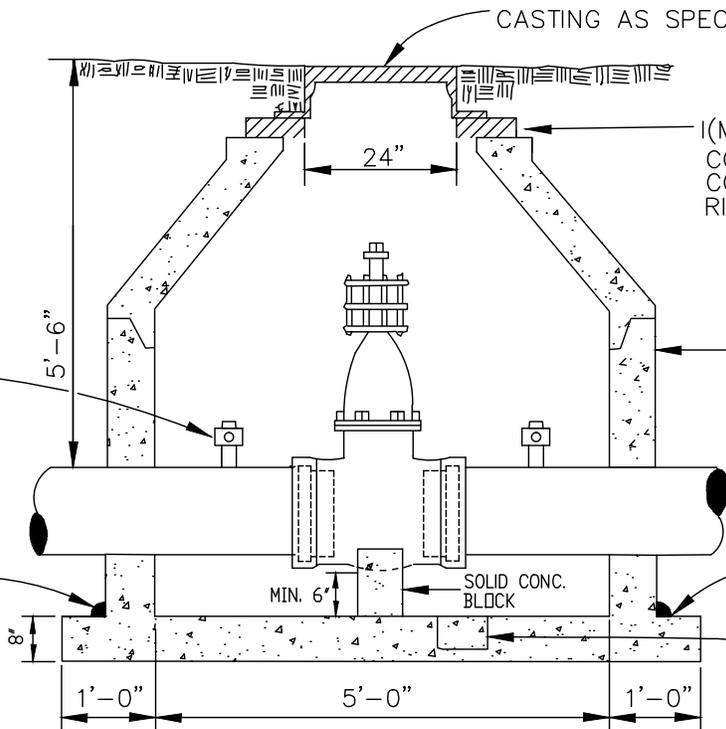
NOTE: ALL LIFT HOLES AND JOINTS SHALL BE MORTARED BOTH INSIDE AND OUTSIDE.
