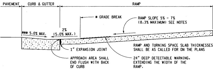
\* GRADE BREAKS AT THE TOP AND BOTTOM OF CURB RAMPS SHALL BE PERPENDICULAR TO THE DIRECTION OF TRAVEL.
