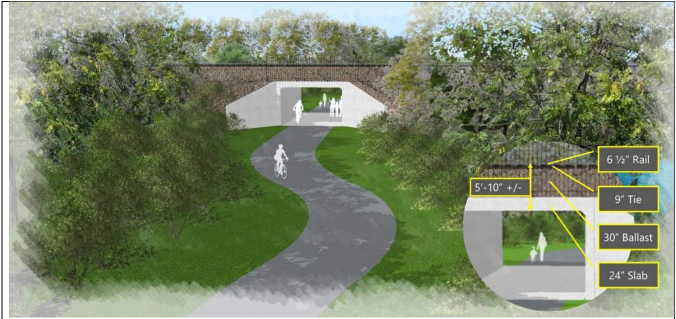
Exhibit 1-11: Box Culvert (ST-1) Looking Towards the Huron River (16-foot wide opening shown)
