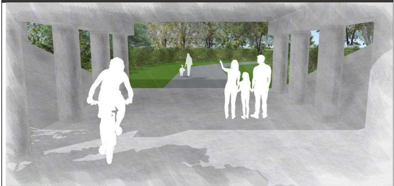
Exhibit 1-16: Rail Bridge (ST-2) Showing a 3-Span Concept from Under the Structure (20-foot wide main span shown)
