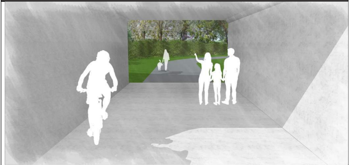
Exhibit 1-12: Box Culvert (ST-1) Inside the Underpass (16-foot wide opening shown)
