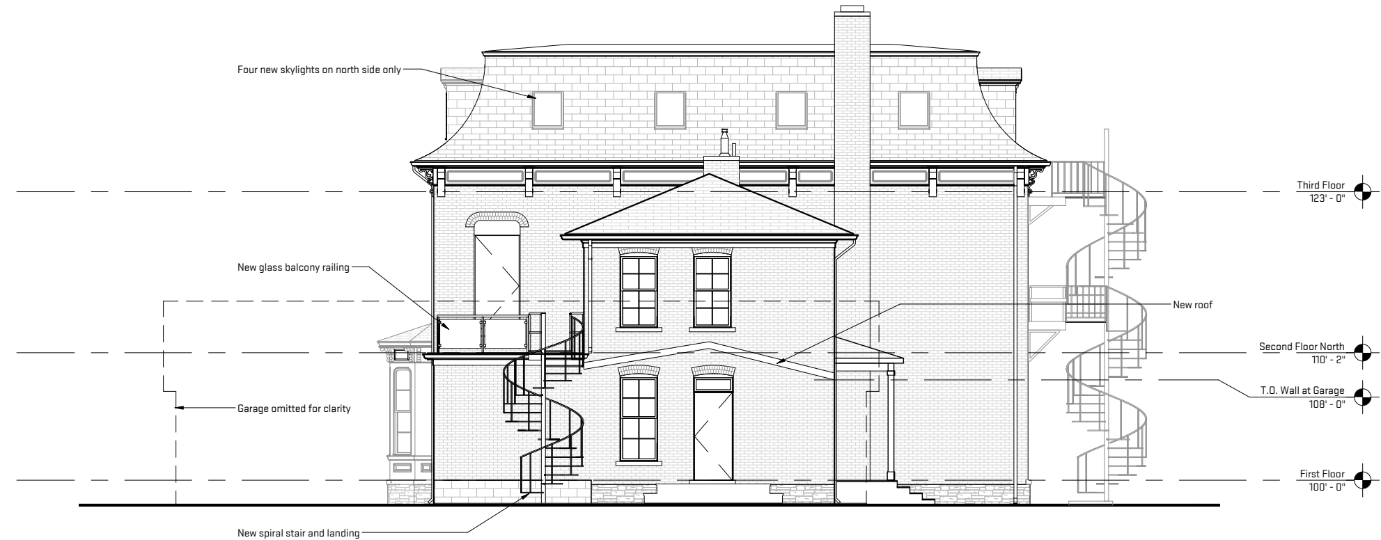
1 North Elevation New Work A-2.2 Scale: 3/32" = 1'-0"
