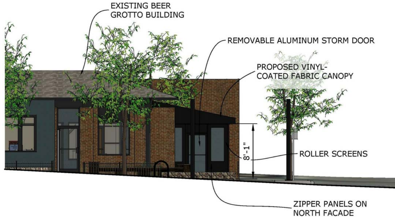
○ NORTH ELEVATION W/ PANELS 1/8" = 1'-0"
