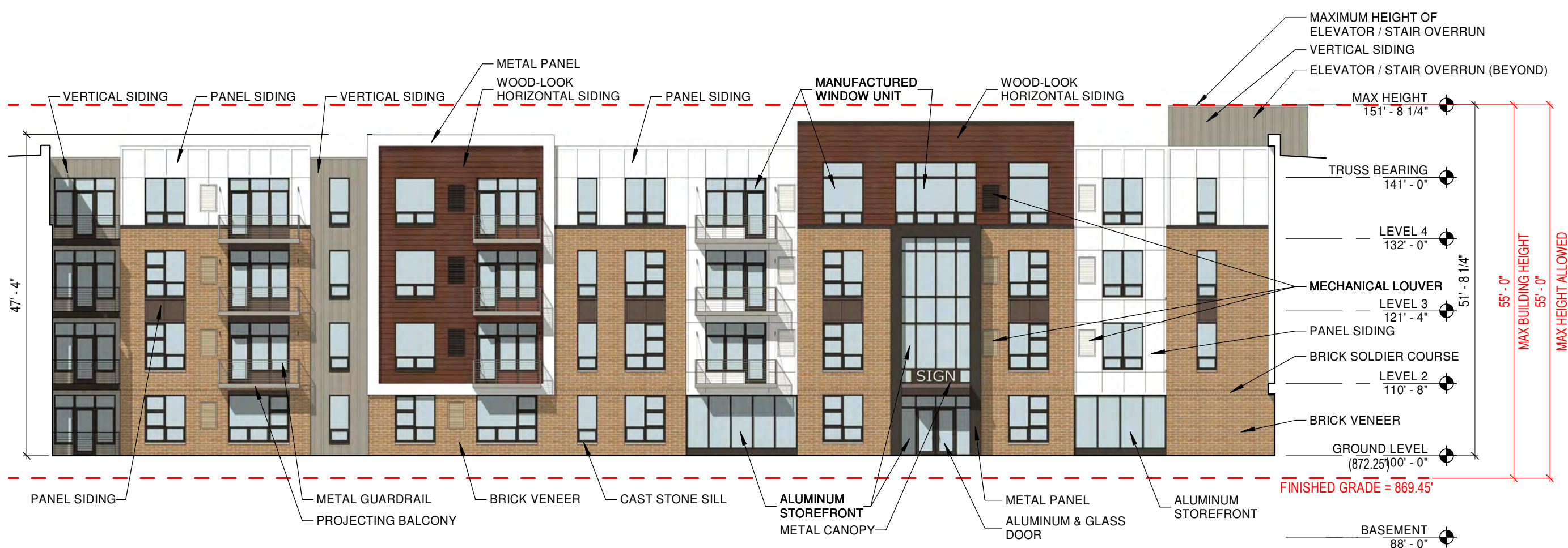
2 NORTH COURTYARD ELEVATION SP-06 SCALE: 1/16" = 1'-0"
