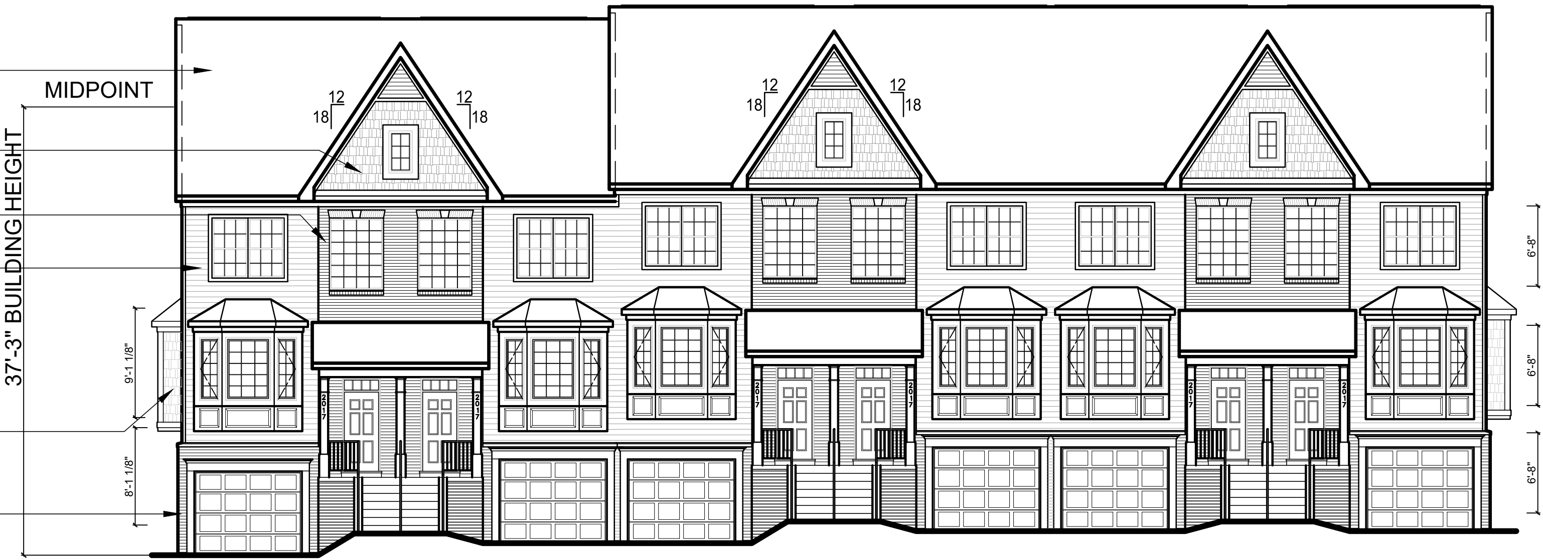
FRONT ELEVATION - BLDG. B SCALE: 1/8" = 1'-0" 6 Unit View-out
