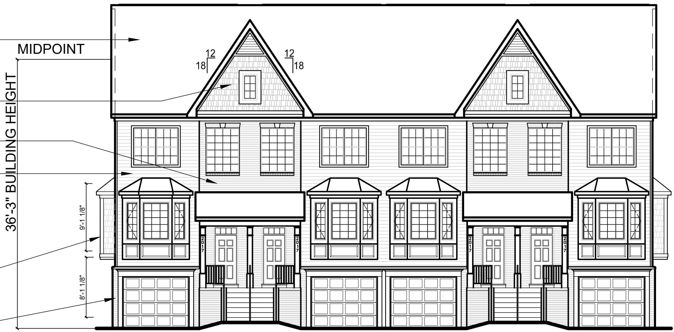
FRONT ELEVATION - BLDG.C SCALE: 1/8" = 1'-0" 4 Unit View-out
