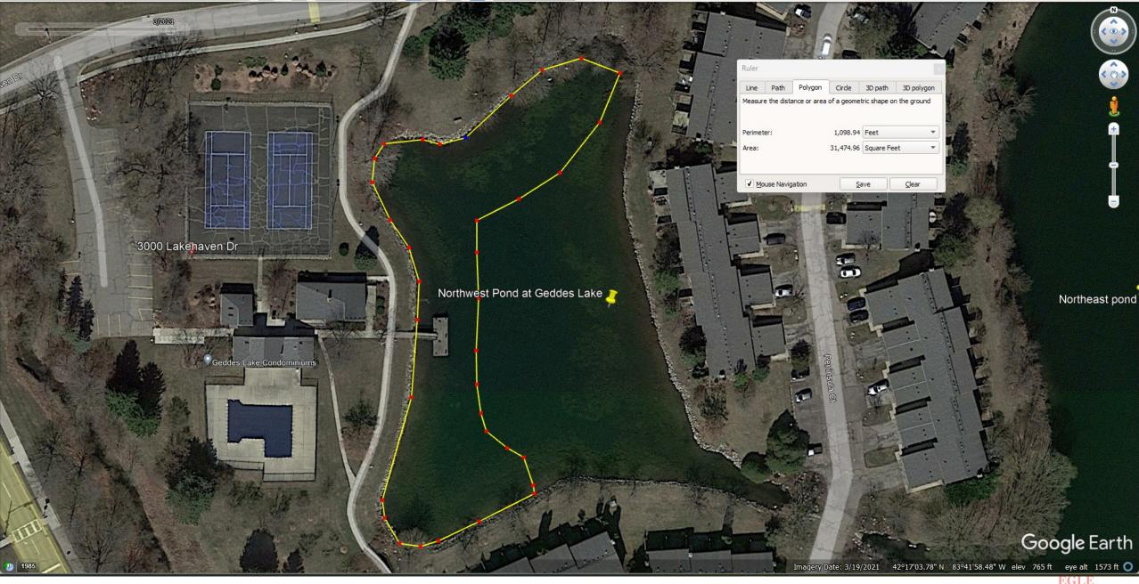
Sketch of the area for sediment removal from the Northwest pond. This area measures 31,474 square feet or 0.72 surface acre. The sediment in this area averages 2ft. The removal of 21 feet of 0 organic sediment from this area will result in the removal of approximately 283 cubic yards dewatered.
