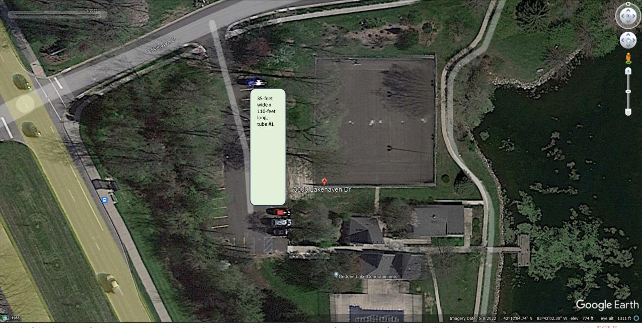
Sketch of the placement of sediment containment tube #1. This sediment tube area will measure 35-feet wide x 110-feet long. It will displace several parking spaces however with lot will be continue to have limited use. This sediment tube will need to lay and dewater for 10 to 12 weeks or until the sediment is dewatered to the point it can be hauled away. This tube will yield ed approximately 200 to 220 cubic yards of dewatered sediment.
