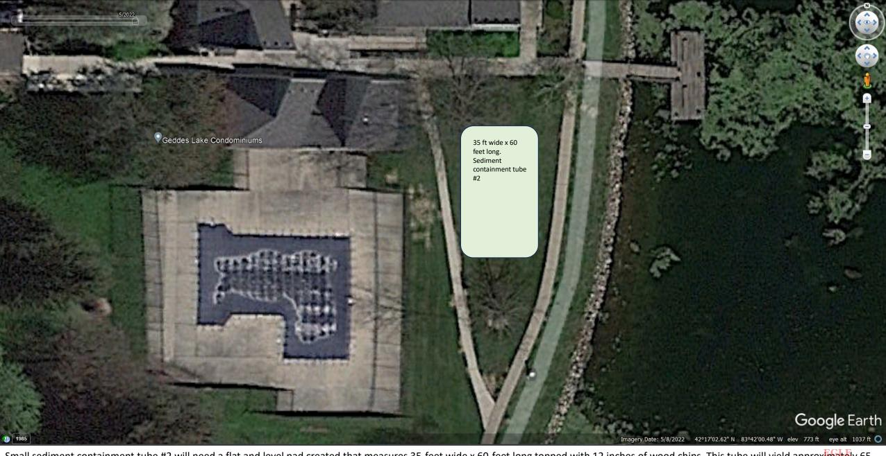
Small sediment containment tube #2 will need a flat and level pad created that measures 35-feet wide x 60-feet long topped with 12 inches of wood chips. This tube will yield approximately 65 to 70 cubic yards of dewatered sediment. Once filled, the sediment containment tube will need to lay and dewater for up to 10 to 12-weeks until it can be hauled away. There is one small dead tree that will need to be removed to utilized this area.
