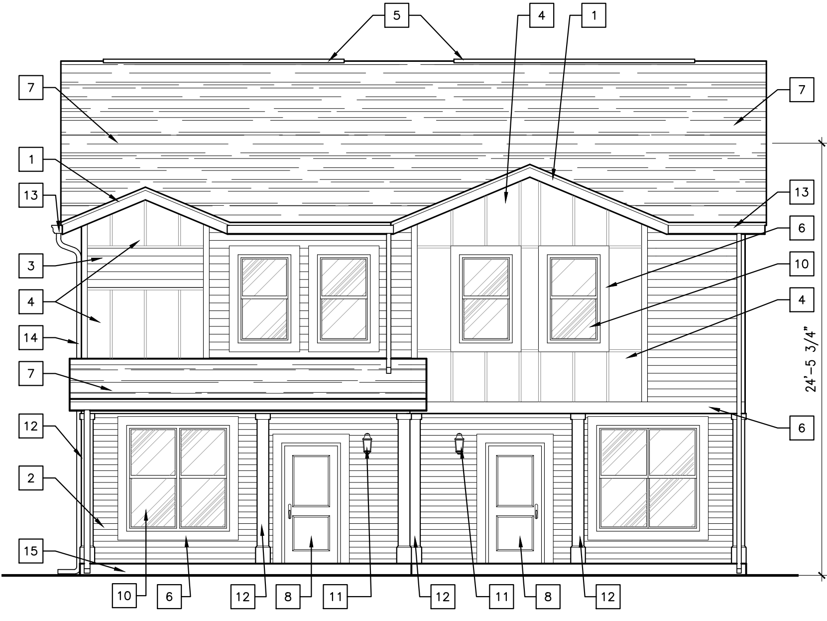
2 DUPLEX 3 FRONT ELEVATION (OPT. A) SCALE: 3/16"=1'-0"
