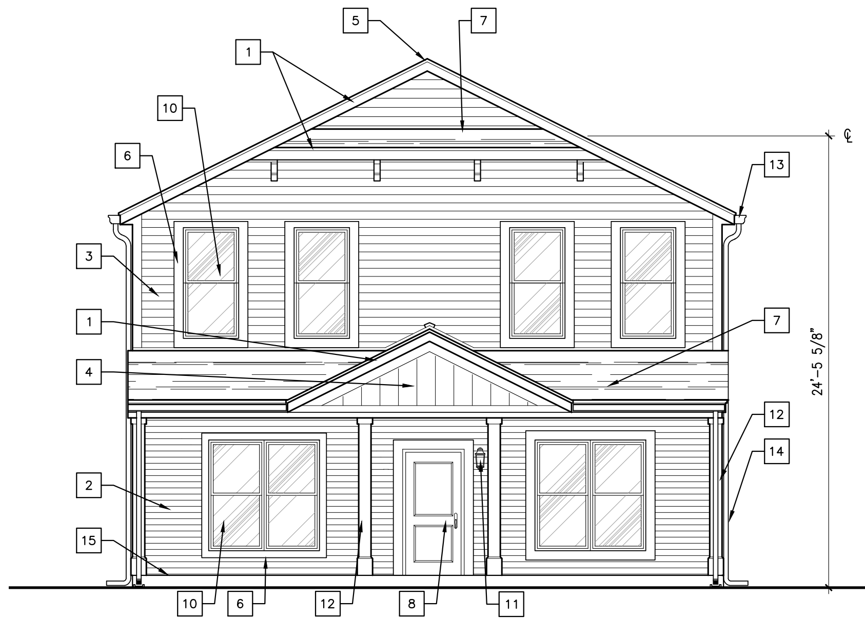
1 A202 UNIT E2 FRONT ELEVATION SCALE: 3/16"=1'-0"
