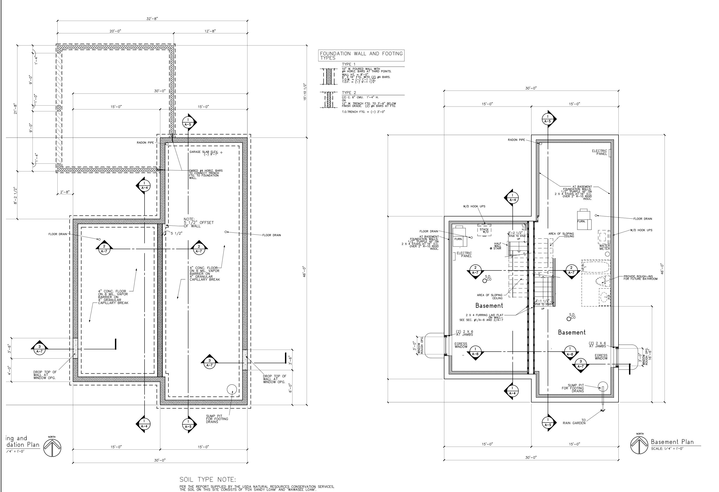
THESE SOILS HAVE A LOAD BEARING PRESSURE OF 2,000 PSF.
