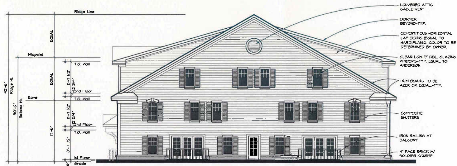
ALT. 'B1' RIGHT SIDE ELEVATION-SOUTH (south building) PITCHED ROOF SCALE: 1/8" = 1'-0" (NORTH BLDG. ELEVATION SIM. BUT OPP. HAND)
