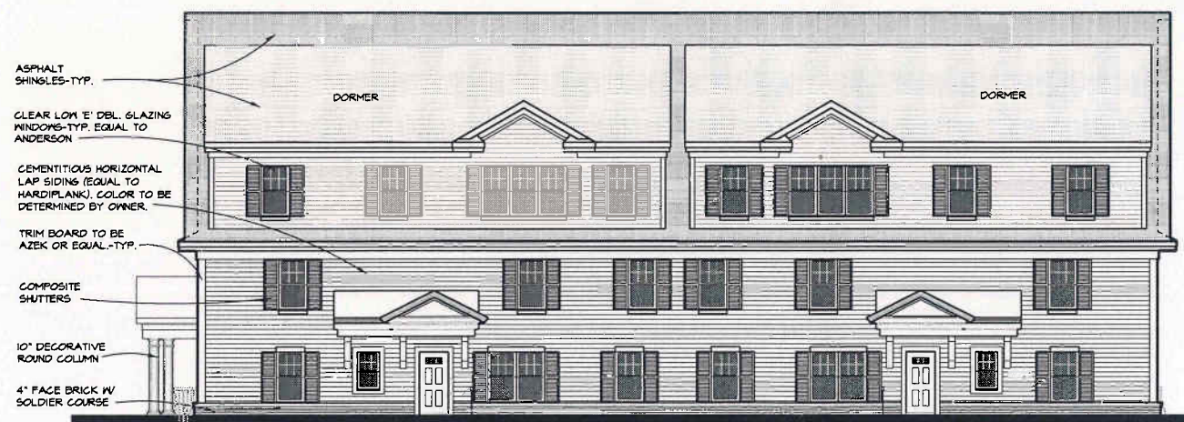
ALT. 'B1' FRONT ELEVATION-WEST (south building) PITCHED ROOF SCALE: 1/8" = 1'-0" (NORTH BLDG. ELEVATION SIM. BUT OPP. HAND)
