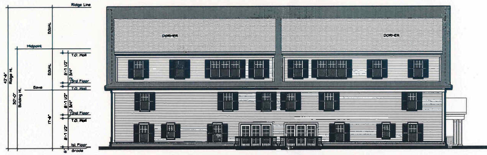
ALT. 'B1' REAR ELEVATION-EAST (south building) PITCHED ROOF SCALE: 1/8" = 1'-0" NORTH BLDG. ELEVATION SHL. BUT OPP. HAND!
