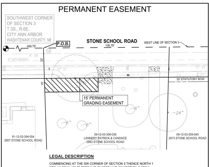
COMMENCING AT THE SW CORNER OF SECTION 3 THENCE NORTH 1 DEG 11' 20" W 459.75 FEET IN THE WEST LINE OF SECTION 3 FOR A PLACE OF BEGINNING, THENCE N 1 DEG 11' 20" W 136.79 FEET, THENCE S 89 DEG 10' 20" E 258.24 FEET, THENCE S 0 DEG 45'40" W 121.68 FEET, THENCE S 87 DEG 26 '40" W 253.97 FEET TO THE PLACE OF BEGINNING, BEING PART OF W 1/2 OF SW 1/4 OF SECTION 3 T3S-R6E 0.76 ACRES.
