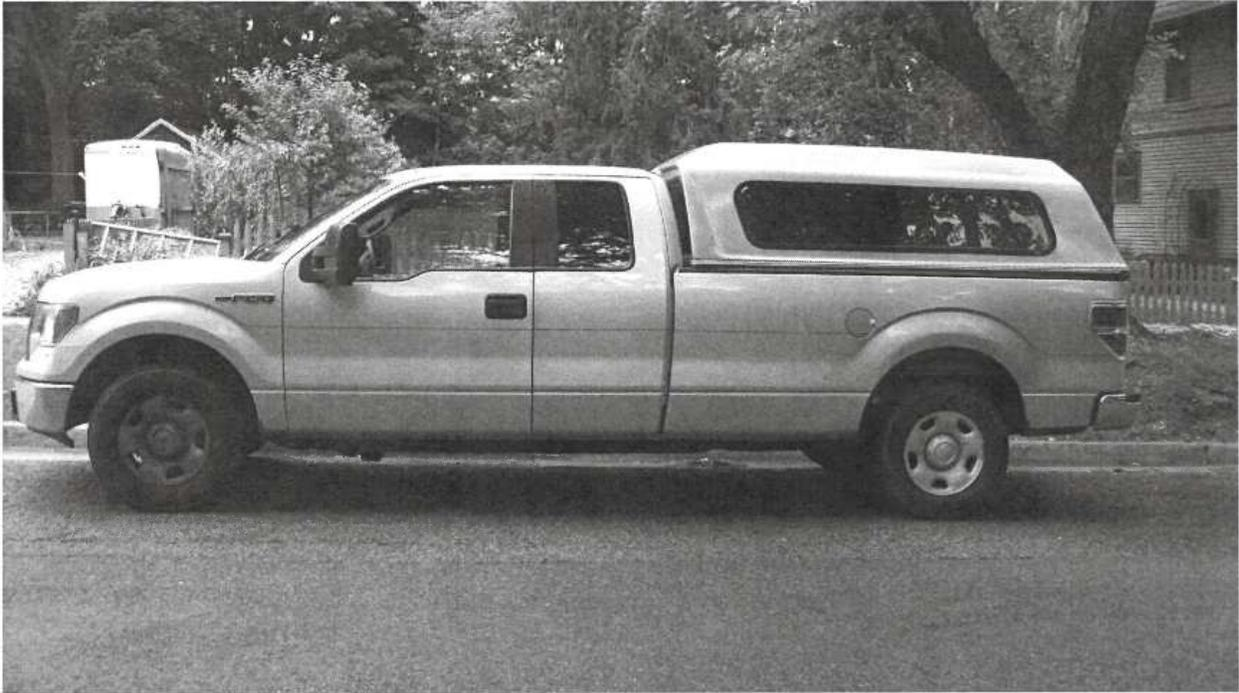
My truck is longer than most — the cab needs to accommodate my family of four, plus dog, in a pinch, and my work needs dictate a full-size, eight-foot, bed. This results in a truck that is over 22 1/2 feet long, with tailgate down. The minimum usable garage depth for the truck alone is therefore about 26-27', which allows for walking around the ends from one side to the other.
