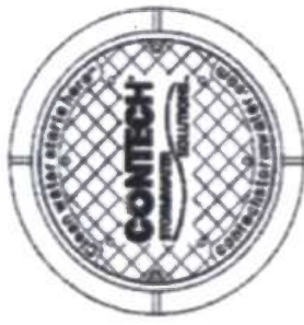
FRAME AND COVER (DIAMETER UNLESS NOTED) N.T.S.
