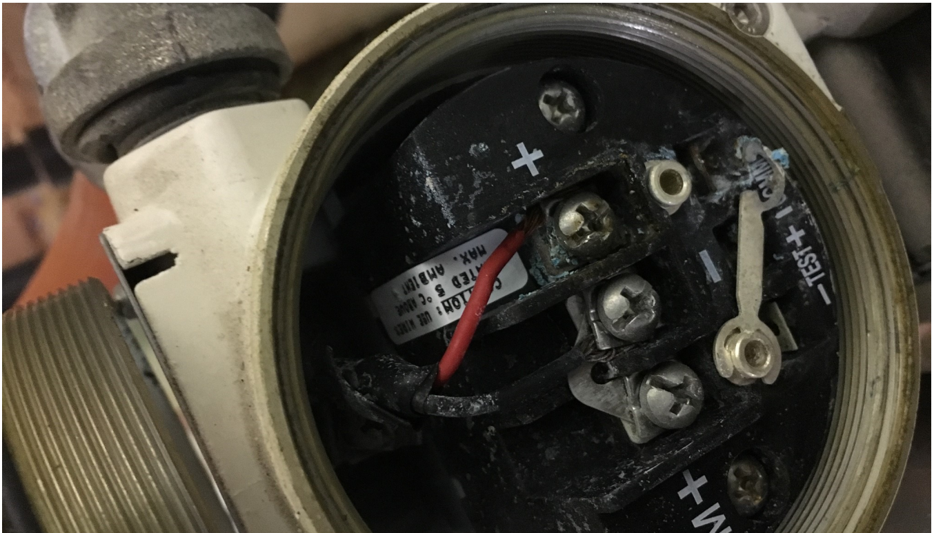
ABB Filter Headloss Sensor. Sensor was immersed and water entered inside of device. Device has failed. Wire terminations are corroding. Typical of 16.
