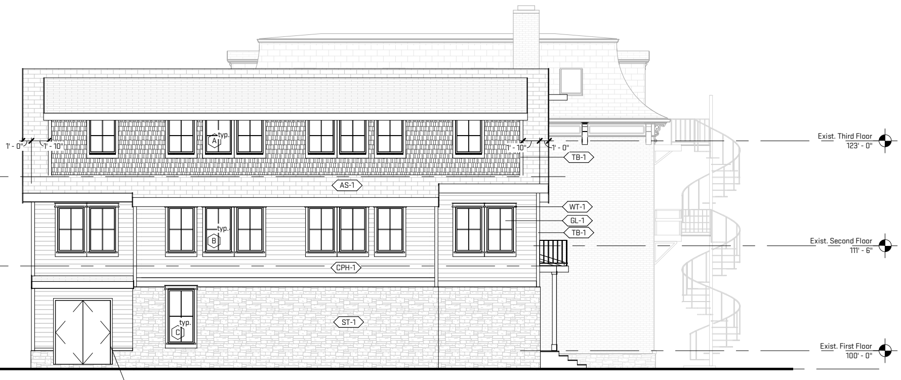
1 North Elevation New Work A-3.1 Scale: 3/32" = 1'-0"
