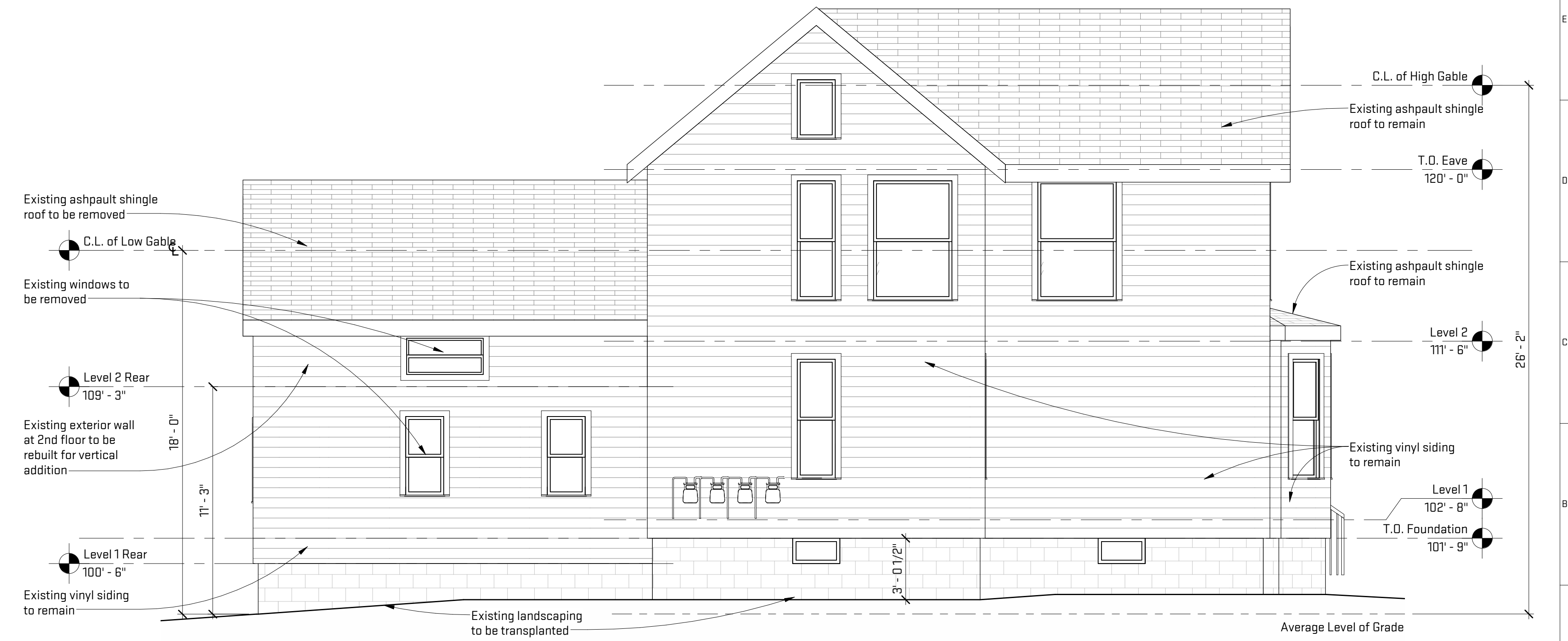
1 Existing West Elevation X-2.0 1/4" = 1'-0"
