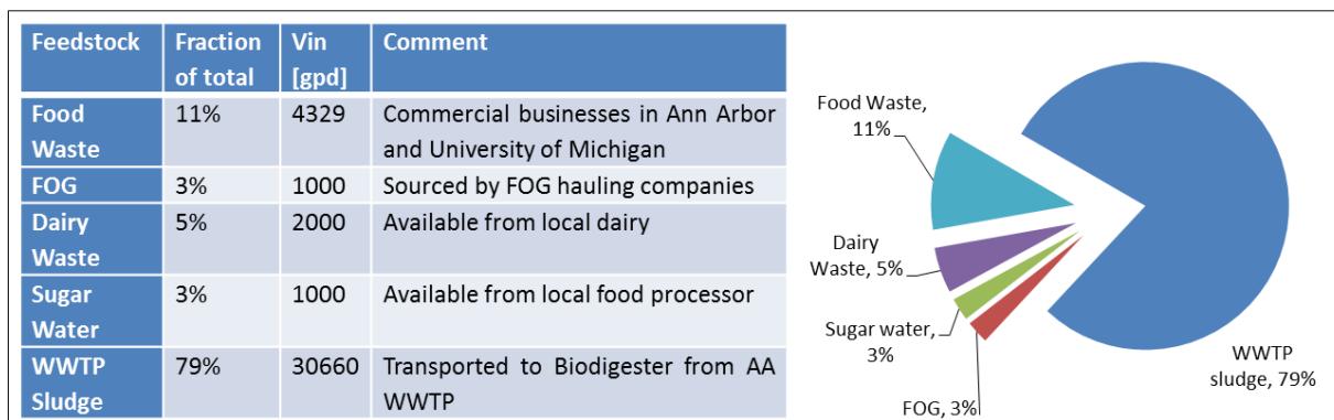
Figure 18: Feedstock menu using 50% of the available WWTP sludge
