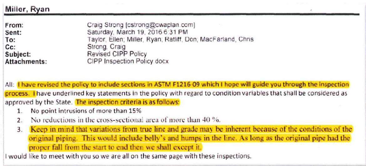
Most pertinent is Mr. Strong’s guidance that “variations from true line grade may be inherent because of the conditions of the original piping. This would include **BELLY’S and HUMPS** in the line. As long as the original pipe had the proper fall from the start to end then **we shall except [sic] it.**” The original email is also attached in Exhibit 8.
