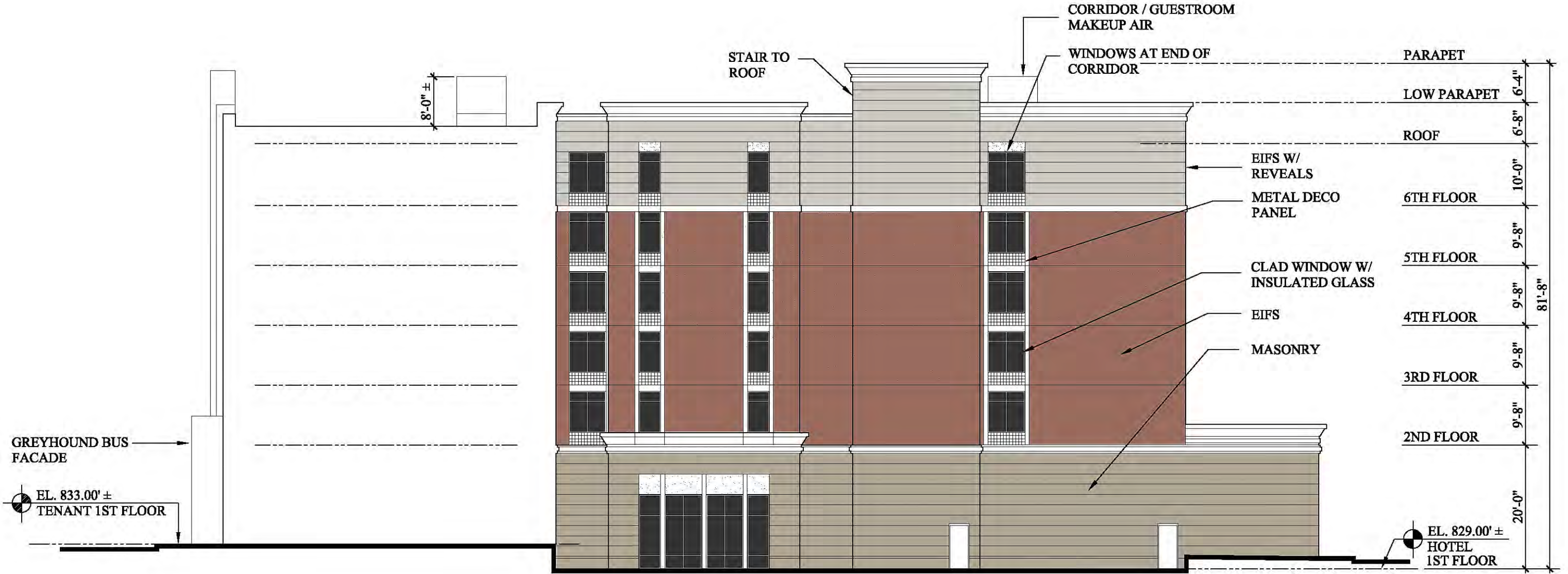
REAR / COURTYARD ELEVATION
