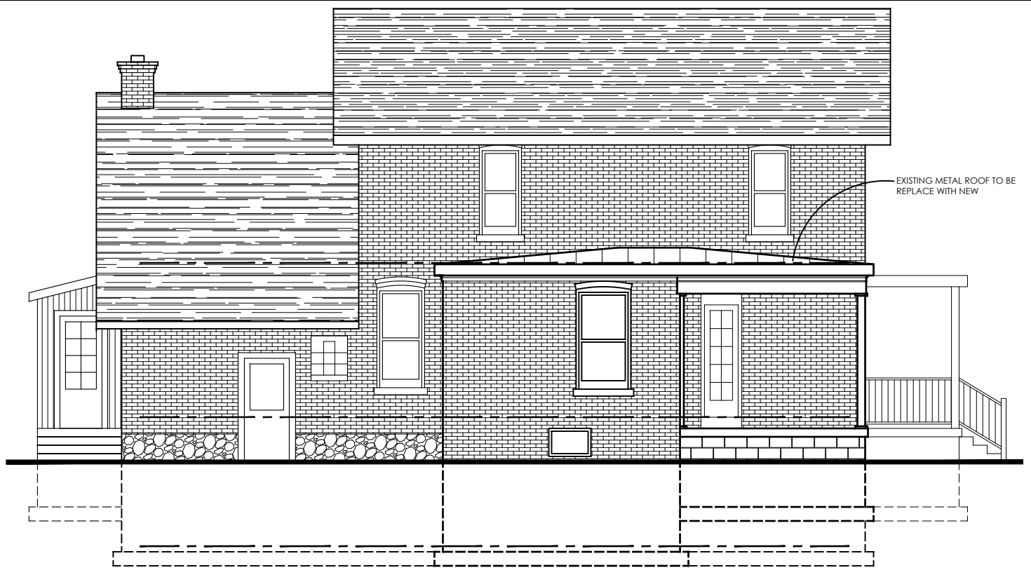
1 EXISTING SOUTH ELEVATION SCALE: 1/4" = 1'-0" ON 22"x34" SCALE: 1/8" = 1'-0" ON 11"x17" & 8-1/2"x11"
