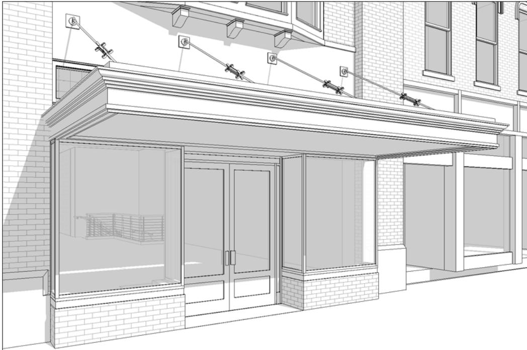
Remove existing plate glass transom window & replace with leaded glass window to match existing -reduce height of window to coordinate with adjacent existing transoms (see historic HDC photo on file)
