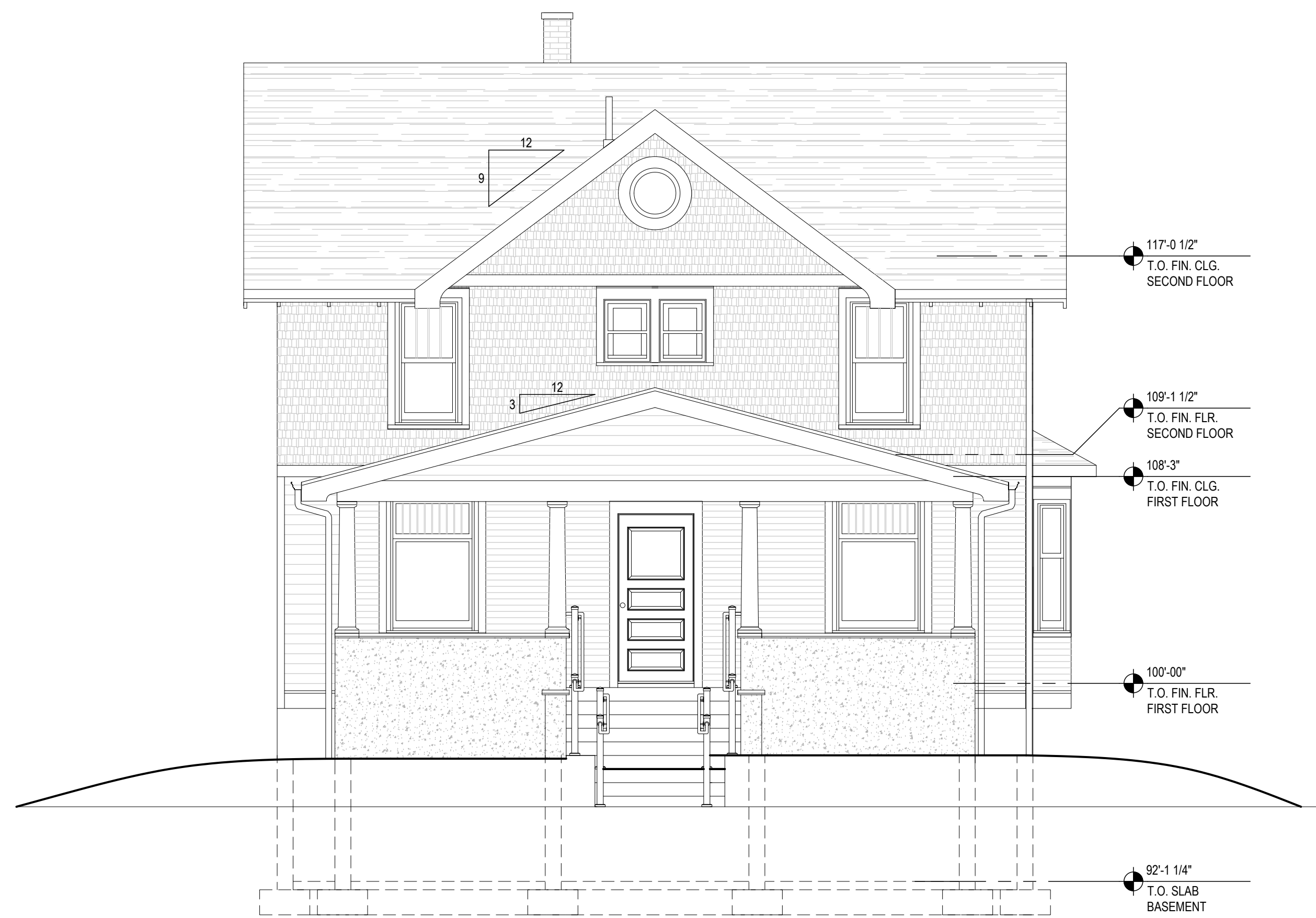
04 Existing East Exterior Elevation SCALE: 1/4" = 1'-0"
