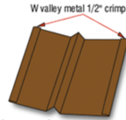
Figure 13d: Roof Valley Flashing Detail
