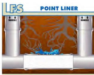
Using our proprietary LFS Point Liner, LiquiForce can repair isolated areas in diameters up to 24" without using disruptive and time consuming excavation methods. Utilizing time proven design principals as per ASTM F1216, we are able to install sectional CIPP liners at any
