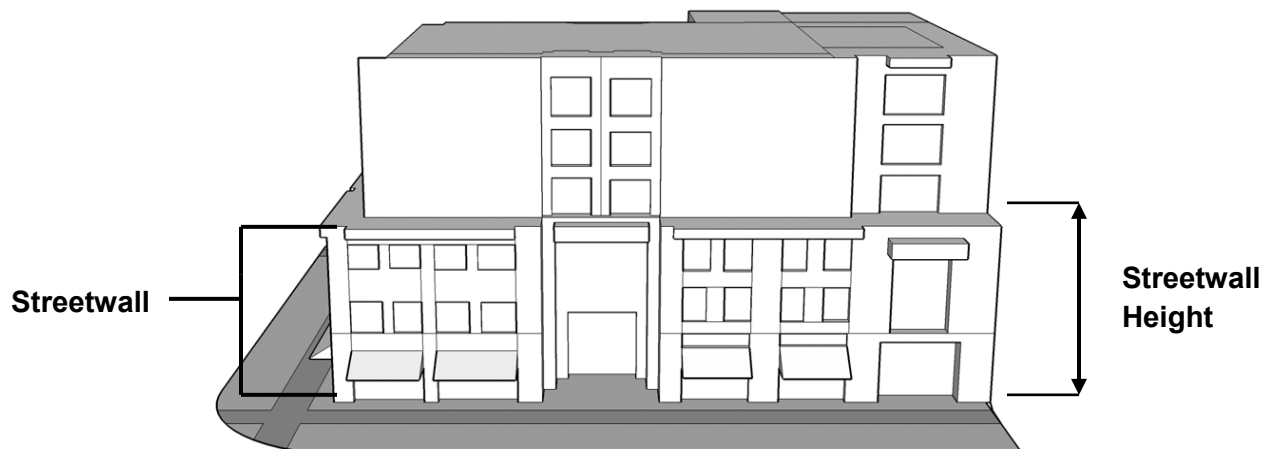
Figure 7: Streetwall and Streetwall Height
