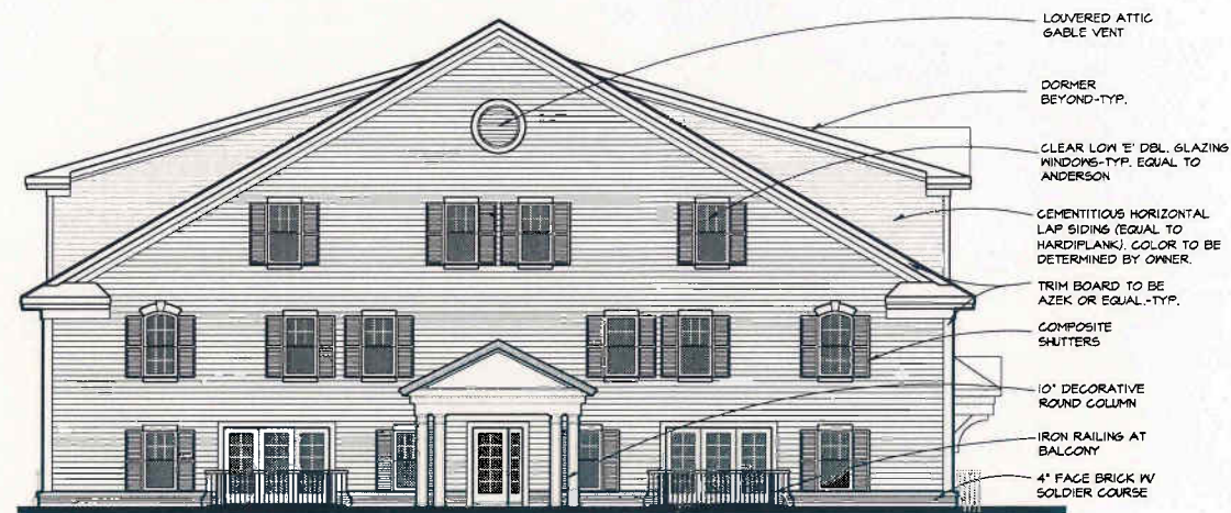
ALT. 'B1' LEFT SIDE ELEVATION-NORTH (south building) PITCHED ROOF SCALE: 1/8" = 1'-0" (NORTH BLDG. ELEVATION SIM. BUT OPP. HAND)
