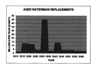
These graphs show that starting in approximately 2016 there is likely to be an increasing need to replace water main pipes within the system. This increase in reinvestment is anticipated to be in the range of 10 times the current rate of replacement. The actual need will be identified as the mains age.
