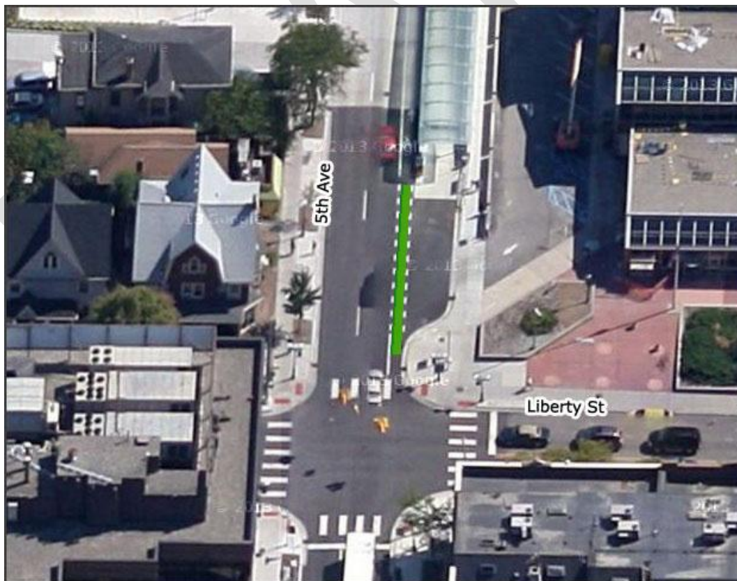
Figure 3 – Green Lane Marking Illustration at S Fifth Ave and E Liberty St – Source: Google Maps and Ann Arbor Staff
