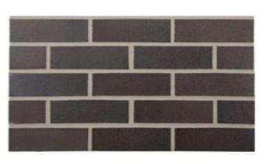
ACTUAL BRICK SAMPLE FOR BUILDING BASE (MORTAR JOINTS NOT TINTED CHARCOAL IN ENDICOT SEINNA IRONSPOT SAMPLE BOARD)
