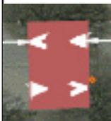
A diagram showing a red-shaded speed table on a road. White arrows indicate traffic flow. The speed table area is highlighted with a red background.
