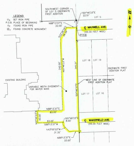
DESCRIPTION OF A PROPOSED VARIABLE WIDTH EASEMENT FOR WATER MAIN
