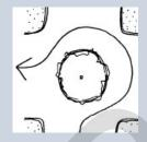
Raised circular islands of pavement, most commonly at four-legged intersections. Does not change existing traffic control, e.g., stop signs.
