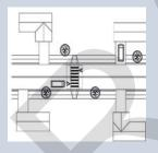
Raised crosswalks are 18 feet wide – including a 6 foot wide center platform marked with crosswalk striping and slopes tapering down on each side, 3 inches high and extend the full width of the street.
